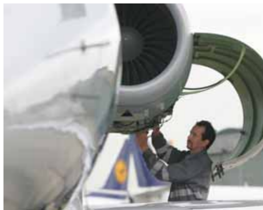
Lufthansa Bombardier Aviation Services GmbH (LBAS) staff servicing the engines of a Bombardier Lear Jet
